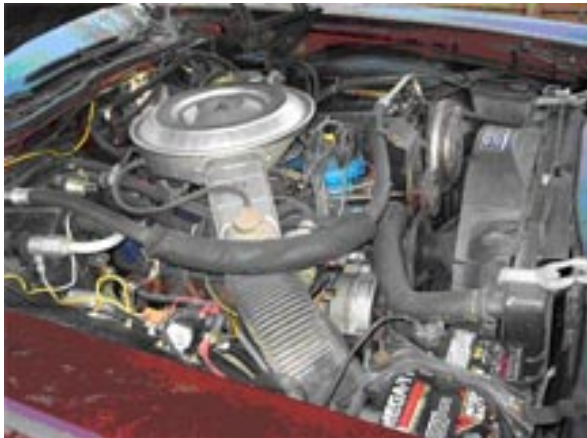
Standard equipment included a rather tame 302 cubic-inch V-8 engine with 129 horsepower and an 8.4:1 compression ratio.
