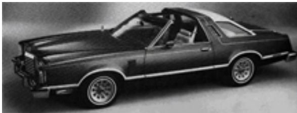
Although a rag top was never offered in this series of Thunderbird models, Ford issued a T-Top option in 1978 to help appease customers who were in the market for a convertible. (Photo courtesy of Illustrated Thunderbird Buyer's Guide )
