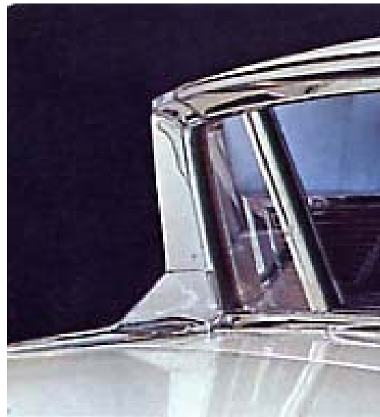
Meteor and Mercury shared the unique Breezeway Window. A power-button option allowed the reverse-cant rear glass to open.
